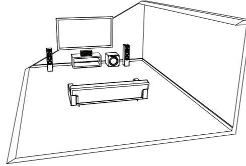
**Front Placement:** In between or to the side of the front channel speakers often results in the best blending with the main speakers and center channel and minimizes localization effects.
