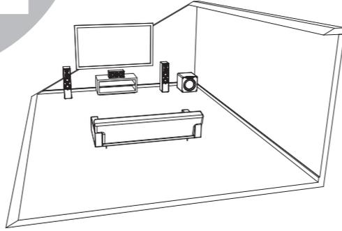
**Corner Placement:** offers huge impact and reduces the potential to encounter bass nulls, or 'dead spots'. If "boominess" occurs, you can try pulling it away from the wall and using the DSP tuning controls to smooth performance.
