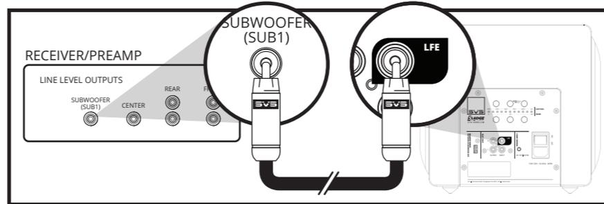
Line Level Connection - Stereo Receiver or Preamp Left/Right Channels
