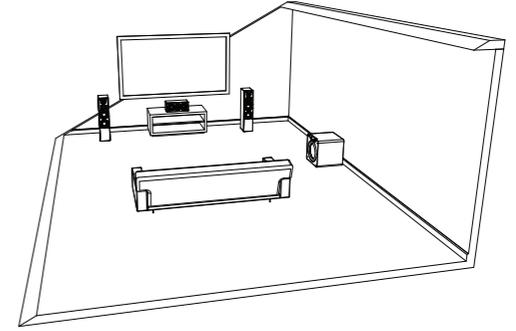
**Side Wall Placement:** Side wall placement is less frequently used but can be an effective subwoofer location for excellent accuracy and output.
