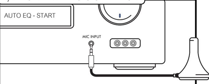
• Run the Auto-EQ setup feature on your A/V receiver. It is important to rerun your receiver's calibration procedure if you are upgrading from another subwoofer.
