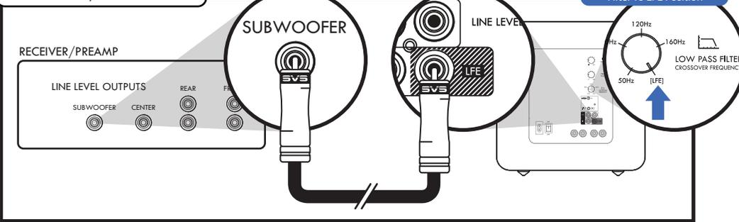
• For most users, the TYPICAL A/V RECEIVER setup is all that will be required to connect your subwoofer.
